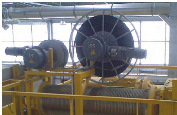
Mono spiral and cylindrical motor driven drums paying vertically down to hook on a special overhead crane.
